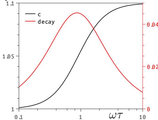
Pic. 15: Phase velocity and decay rate of disturbances in gas with relaxation
