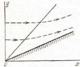
Pic. 7: Streamlines of the flow past a cone
