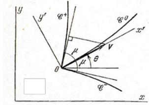
Pic. 5: Geometry of characteristics
