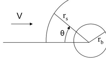
Assume also  $M \gg 1$ . The bow shock in front of the sphere is strong near the axis of symmetry and the gas density after it is close to the limit one and approximately
